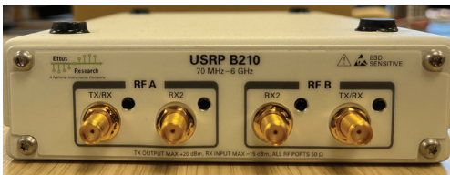
An NI USRP B210 software-defined radio modem
