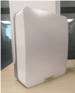
Massive MIMO-based channel sounder
